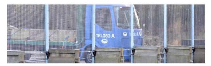
BSi PAS 68 is the a Publicly Available Specification for vehicle security barriers and fences. It has become the standard and security benchmark for Hostile Vehicle Mitigation (HVM) equipment and is the specification against which the perimeter security equipment is tested to prevent vehicle borne attacks.
